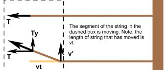
The diagram illuminates the similar triangles involved, where v' is the vibrational velocity and v is the wave velocity.
